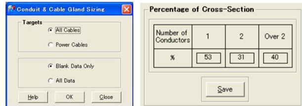
The image shows two dialog boxes. The first, 'Conduit & Cable Gland Sizing', has radio buttons for 'All Cables', 'Power Cables', 'Blank Data Only', and 'All Data'. The second, 'Percentage of Cross-Section', shows a table for conductor counts and their corresponding fill percentages.
