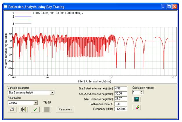
Ground reflections can be analysed by a series of successive ray tracings. The reflecting surface of the entire profile will be covered and represents a more realistic presentation of the reflection characteristics of the path. The relative receive signal can be plotted as a function of the following parameters:
