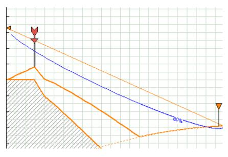
The isolated obstacle algorithm can be used to consider several closely spaced obstructions as one effective obstacle. In the example shown on the right. The loss will be calculated at the arrow location using the radius which encompasses two obstacles. This type of analysis is useful to resolve ambiguities which may arise in the results.
