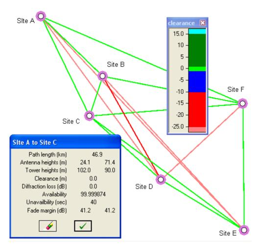
An example of automatic link design for 6 sites is shown above. Links between every combination of sites have been created and designed in one step. The links have been color coded based on the relative clearance of the antenna heights to the design criteria is used. Rejection criteria are used to selectively remove links to arrive at the final configuration.
