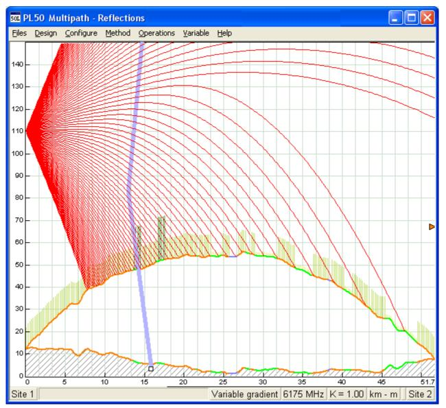
A variable gradient ray trace is carried out to determine the susceptibility of ducting on the path. In the above example the a surface duct M profile results in a space wave fadeout on the path. The program includes the ITU-R P.453-8 ducting data base for surface and elevated ducts along with the probability of occurrence. The M profile is determined using the path center coordinates.
