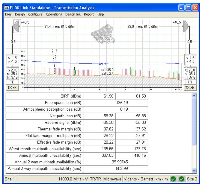
The *Transmission analysis* design section is the data entry point for all radio, antenna, transmission line, antenna coupling unit and frequency assignment data. Each icon on the display brings up the respective data entry form. Data entry can be carried out using lookup tables, data file indexes or by importing data from an existing file. All calculations are automatically updated as the date is entered or changed.
