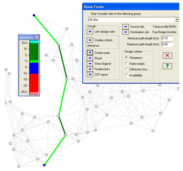
the start and end point and the design criteria and clicked the create route button. Every possible link is analysed within the constraints of the maximum and minimum path lengths. The best route is displayed color coded according to the design criteria, - An extremely powerful feature included in the basic program (PL5B)
