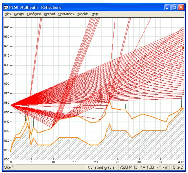
A constant gradient ray trace is used to determine if the path profile geometry can support a specular reflection. This condition is produced when the reflected rays over some portion or the profile arrive above and below the receive antenna. A specular reflection is possible in the example above and would required further analysis. This can be carried out by using a reflective plane or successive ray tracing techniques to quantify the effects of the ground reflections.
