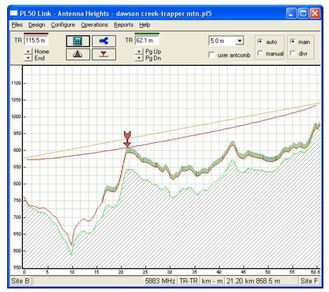
The Antenna heights design section provides an interactive screen display of the path profile and the user's clearance criteria. In the Auto mode, either antenna height can be varied and the other antenna height will be automatically recalculated to meet the clearance criteria. On space diversity applications, the user can switch between the main and diversity antennas,
