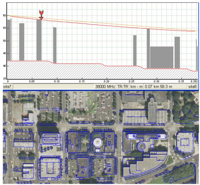
Mapfiles or shapefiles which contain building outlines and building heights, can be configured to be used as clutter data. The path profiles will include the building data. The network display shown below has a backdrop geo refer-
