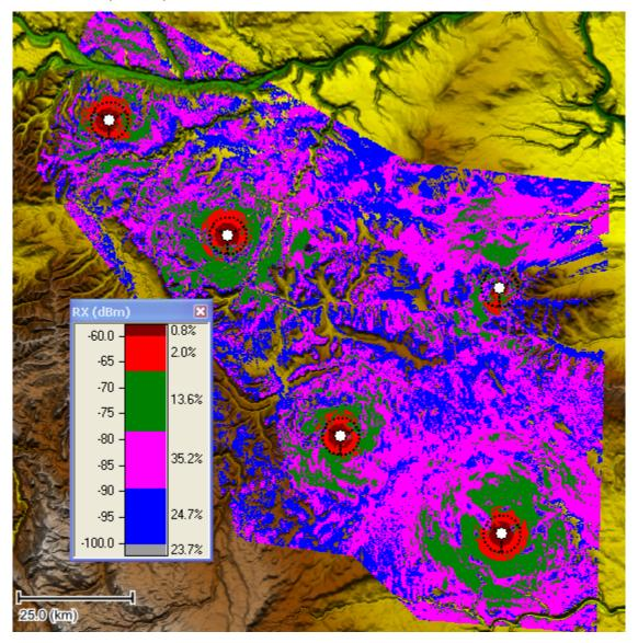
In an area study a common area is specified for all base stations. This coverage area can be a rectangle, ellipse or polygon as shown in the above network display example. The coverage area is divided up into uniform cells. The signal strength from each base station is calculated into each cell in the coverage area.
